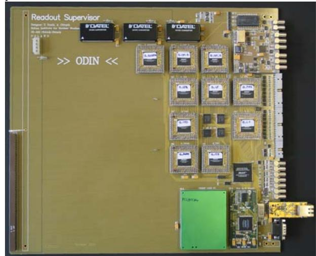
Fig. 6. The first prototype of the Readout Supervisor has been built and tested successfully.
