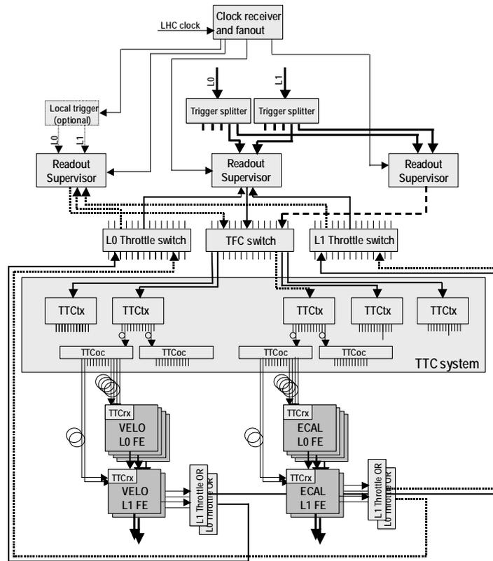
Figure 1: Overview of the TFC system architecture.
