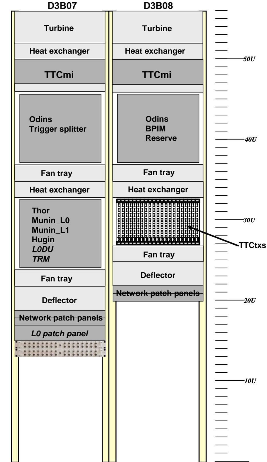
Figure 3: A schematic view of the TFC racks.
