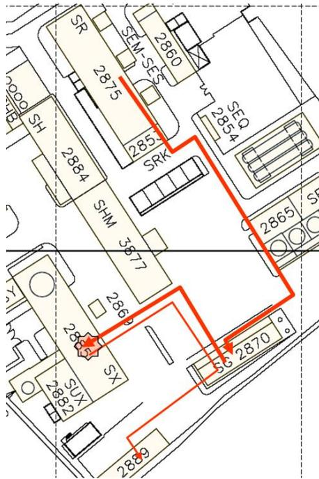
Figure 2: Routing of the fibres between SR8 and SX8.
