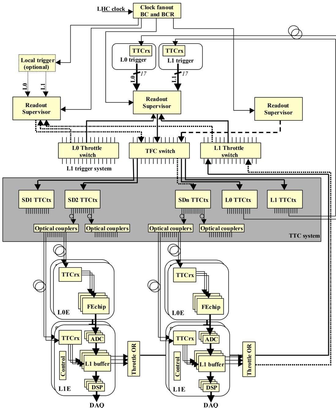
Figure 1 General Architecture of the LHCb TFC system
