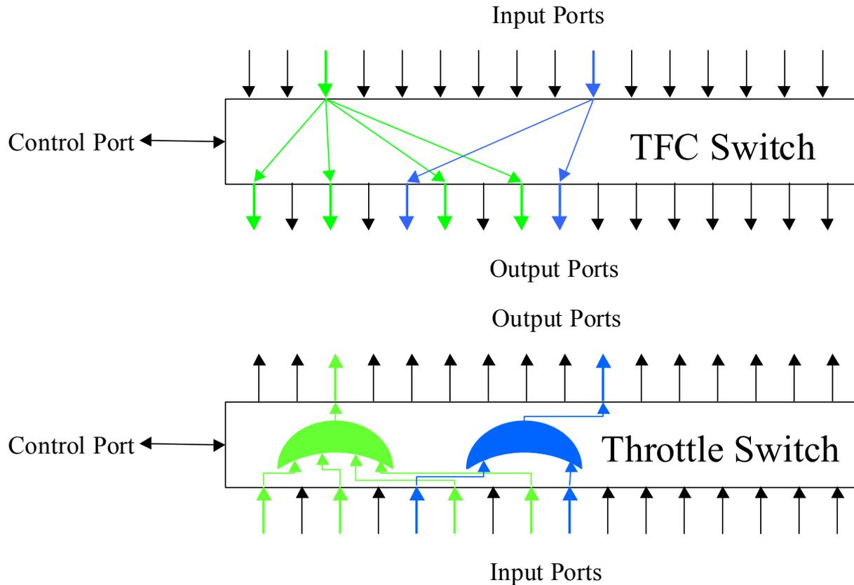
Figure 2 Schematic diagram of the external interfaces the TFC switch (upper diagram) and the Throttle switch (lower diagram) implement.
